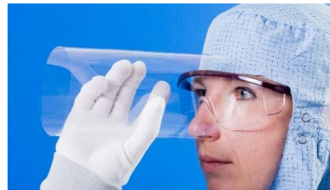
Glass with a thickness below 100 \mu\text{m} is flexible
